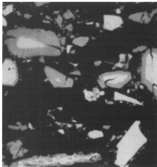
Fig. 1 Photomicrograph of AQUANIDE Nd-Fe-B powder with passivated surface layer.
